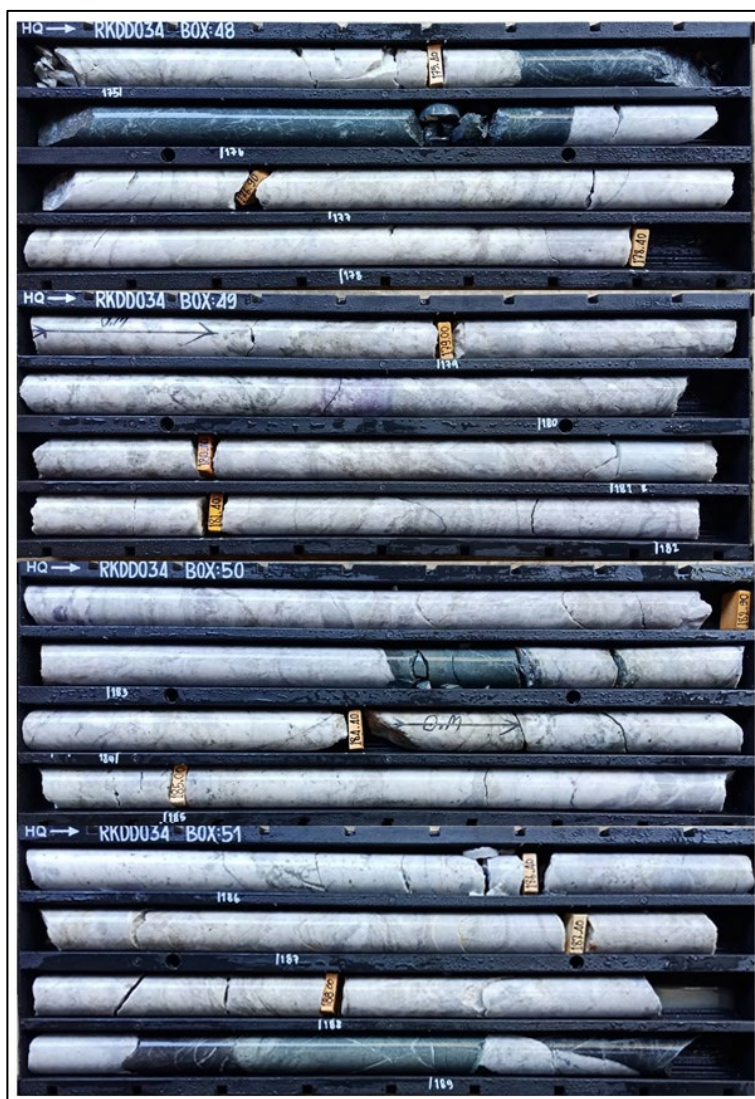
Photo 1. RKDD034 from 174.9m to 189.3m, showing part of upper pegmatite
