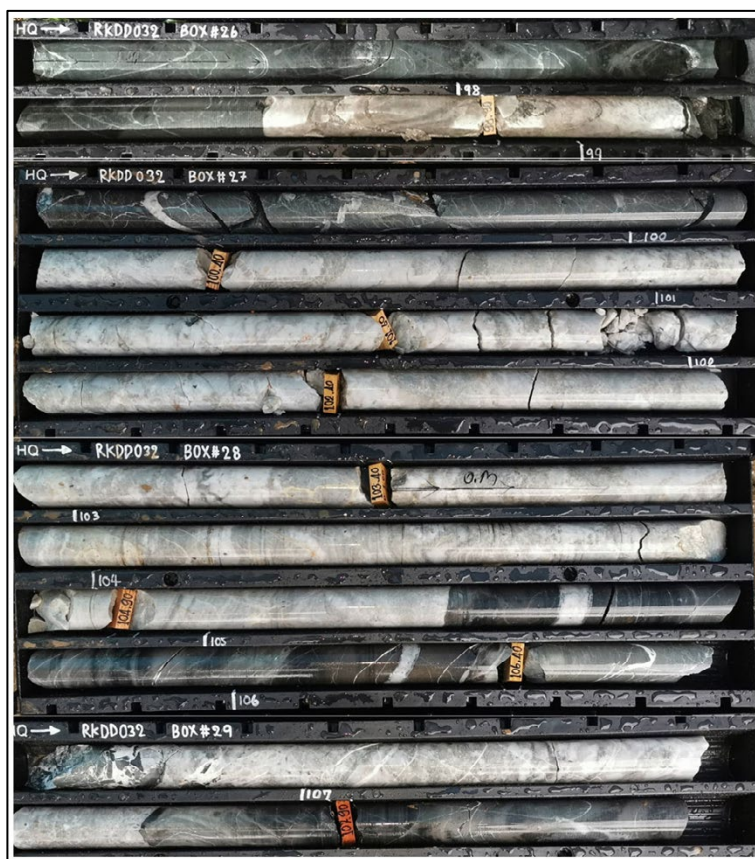
Photo 4. RKDD032 from 97.4m to 108.2m, showing pegmatite swarm with pale lepidolite.
